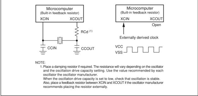
Figure 7.10 Examples of Sub Clock Connection Circuit
